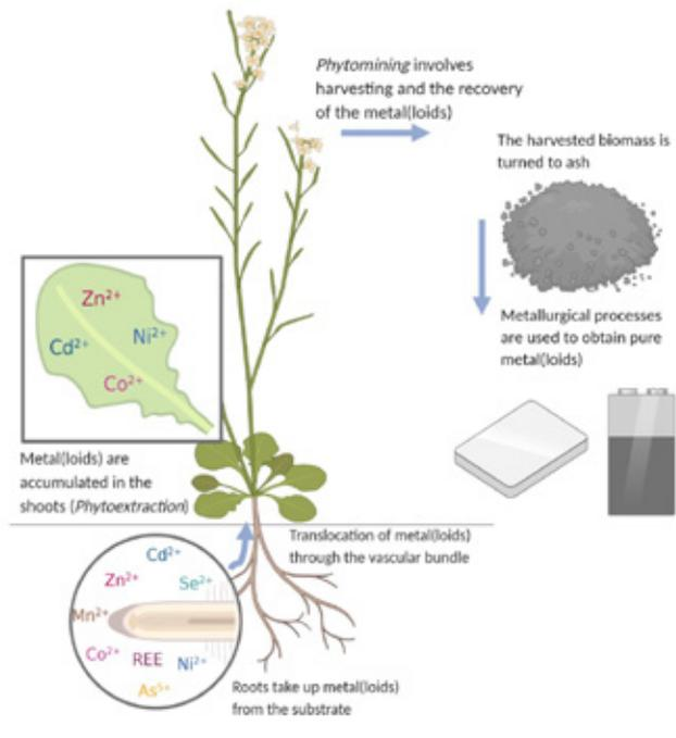
Figure 14. Main processes in phytomining. Figure created in Biorender.com and Mind the Graph platform.
