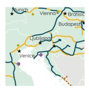
Plinovodi, the TSO of Slovenia, operates a network of 1,195 km, for domestic use while also playing a transit role from Austria to Croatia and Italy. For both using a doubled main backbone from its capital Ljubljana into the east which then stretches north into GCA's and TAG network in Austria. With the LNG terminal in Croatia on the Krk Island, up and running since the beginning of 2021, the new planned
