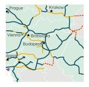
FGSZ, Hungary's gas grid operator, operates a mature network of 5,874 km. The network is partially for domestic use, while playing a recently changed transit role from Ukraine to south-eastern Europe. The flows reversed partially and decreased slightly with opening of the LNG terminal on the Croatian island Krk in 2021 and with the gradual opening of the new Balkan routes. Therefore,
