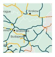
EUSTREAM's transmission system in Slovakia represents an important east-west and north-south energy connection. A robust system of 4 to 5 parallel pipelines is connected to the primary transmission routes in Ukraine, Hungary, Austria and Czech Republic (a new gas interconnector with Poland will be commissioned soon).
