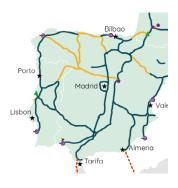
Enagás operates an extensive gas transmission network in Spain that comprises over 11,000 km of gas pipelines. This network has six international connections: two with Africa via Tarifa and Almeria (linking with the Magreb and Medgaz gas pipelines, respectively); two with Portugal via Badajoz and Tuy; and another two with France via Irun and Larrau. The Spanish Hydrogen Roadmap
