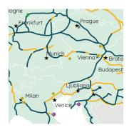
Austria's current transmission gas network is operated by two TSOs, TAG and GCA and stretches over ~1,700 km. TAG mainly transits natural gas from the eastern border with Slovakia towards Italy. GCA's network serves a dual function and simultaneously transits gas mainly from Slovakia towards Germany, Hungary and Slovenia and provides gas via its primary distribution system for domestic customers in Austria.
