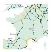
France's current gas network is operated by GRTgaz which operates 32,000 kilometres of pipelines and Teréga, which operates a 5,000 km network in the South-West. The networks serve industry, power and residential customers while GRTgaz also transits gas to Switzerland, Italy, and Teréga transports gas to and from Spain, connecting the Iberian peninsula. Both TSOs
